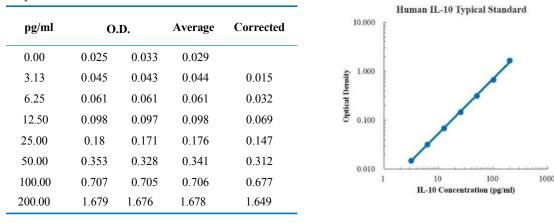
A standard curve must be run within each assay. This standard curve is provided for demonstration only.
